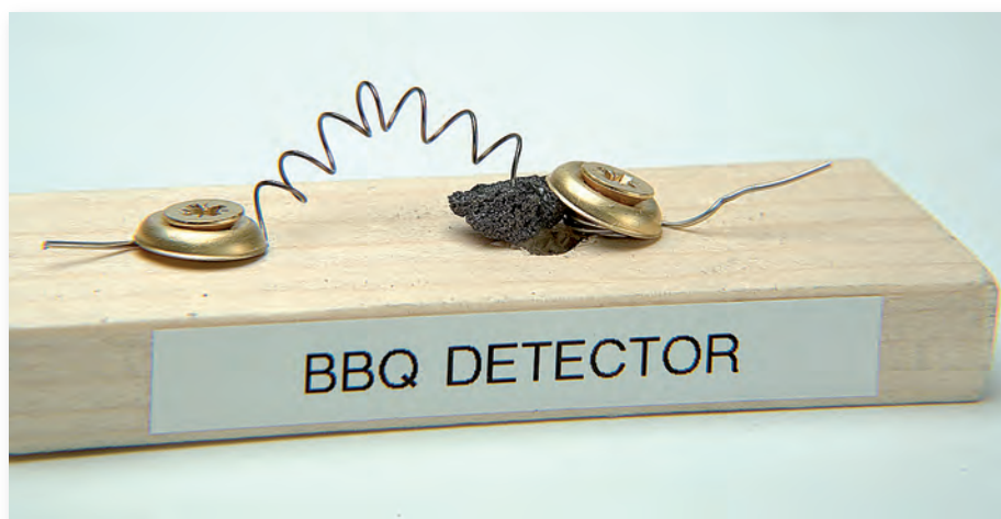
Fig. 5: Using a piece of coke as the 'crystal' with a cat's whisker.
