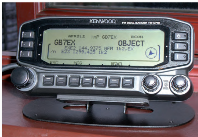
Fig. 3: The '710E acts as a stand-alone Packet Radio unit.
