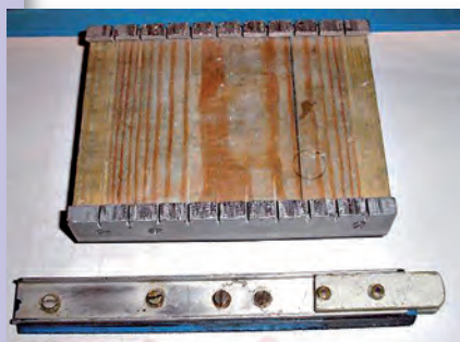
Fig. 2: the metal-sided jig and hacksaw blade (held in two lengths of aluminium for support) for cutting the copper-cladding of the p.c.b. material.
