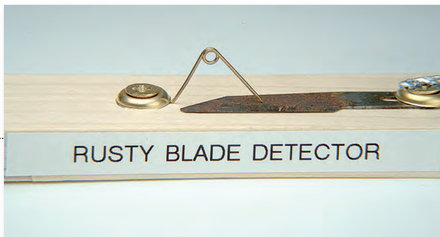
Fig. 4: As used in Prisoner-of-war camps, the rusty blade detector.
